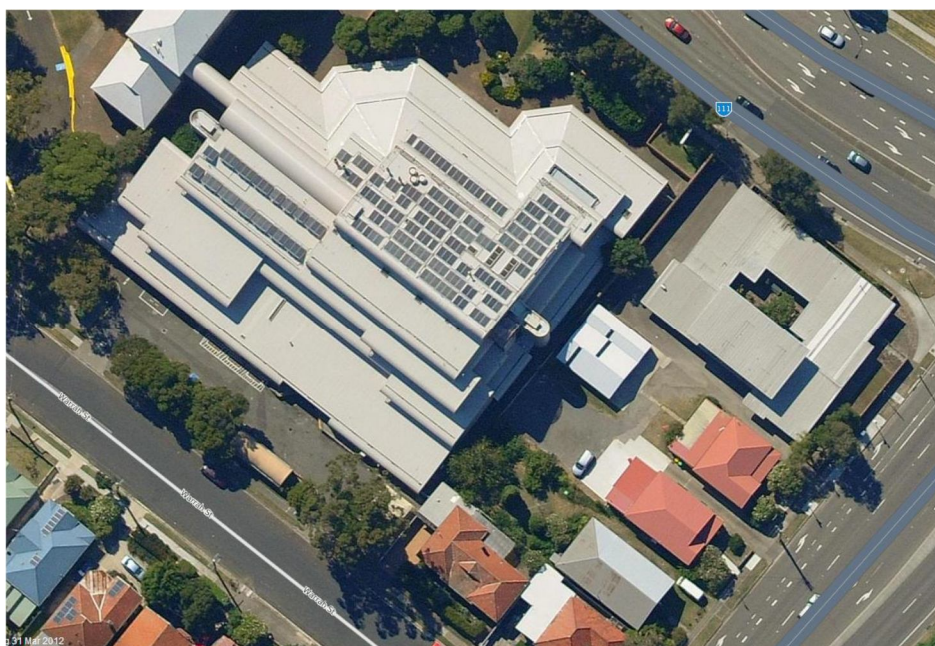
Figure 38: Aerial view of Hamilton TAFE building showing solar collectors on the roof
